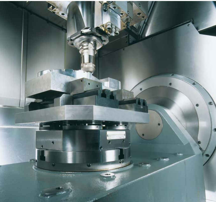
Precision rotary / tilting tables achieve maximum performance thanks to bearing solutions supplied by INA and FAG
