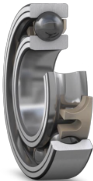
Deep groove ball bearing for cryogenic pumps, featuring VC4444, a special variant of SKF stainless steel, as well as low-friction ceramic rolling elements
