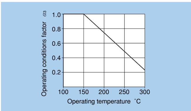
Fig. 3.2 Operating conditions factor according to operating temperature
