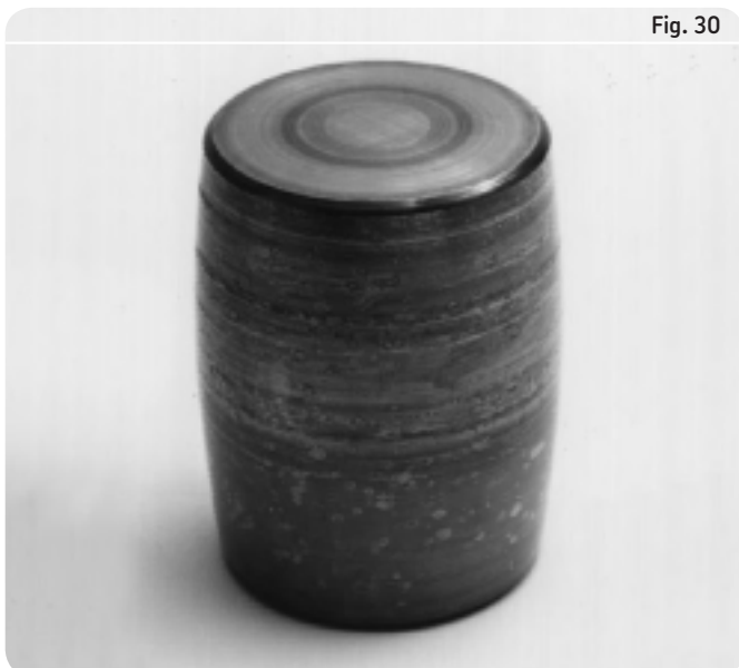
Figs 30 and 31: Smearing normally leads to premature spalling
