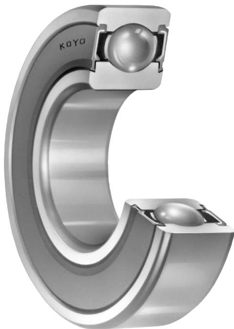
Koyo produces shielded ball bearings and sealed ball bearings of non-contact type (Z and RU types) and contact type (RS and RK types). In general, non-contact type products are used in applications requiring low torque, and contact type products in applications requiring tight sealing.
