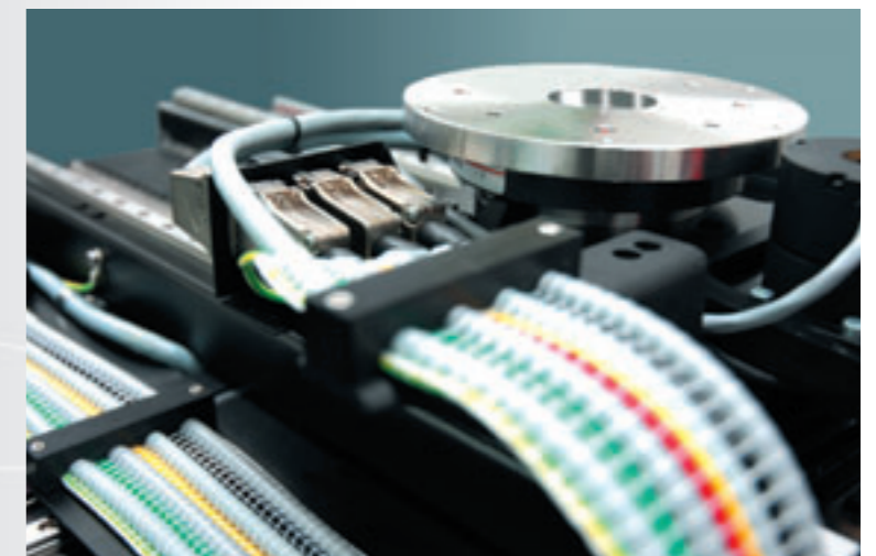
Woven cables for clean-room compatibility
