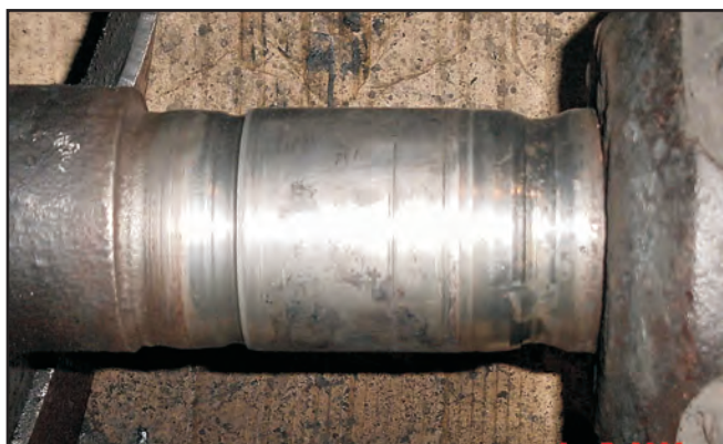
Above: Typical annual shaft damage prior to conversion.
