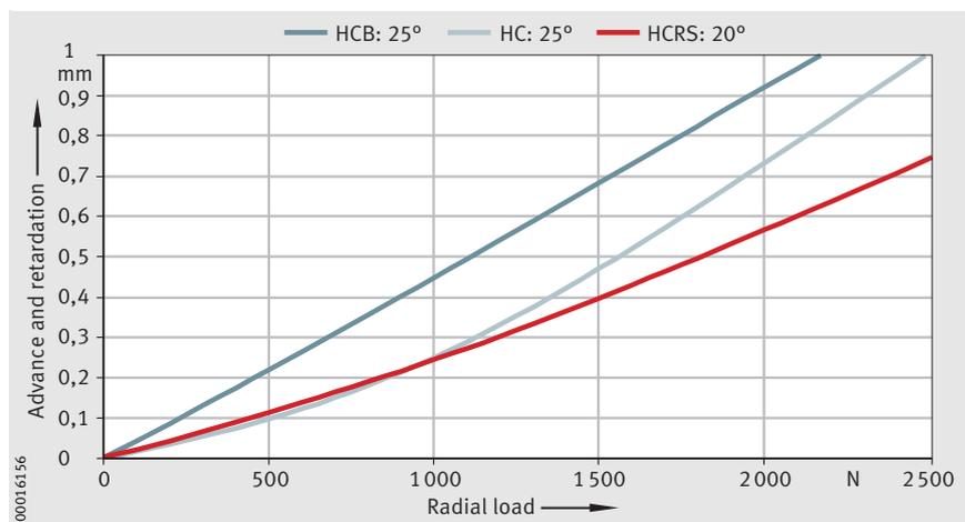
Figure 4 · Advance and retardation due to radial load
