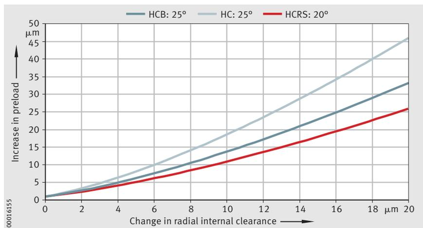
Figure 3 · Increase in preload with changes in radial internal clearance
