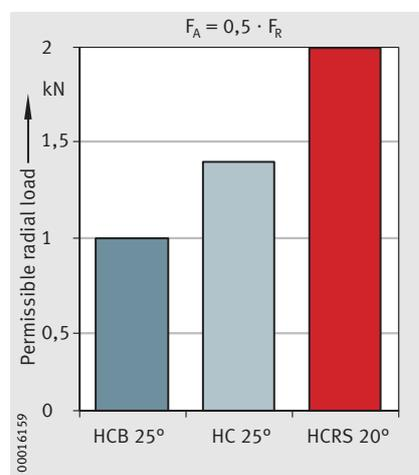
*Figure 7* · Permissible loading under combined load
