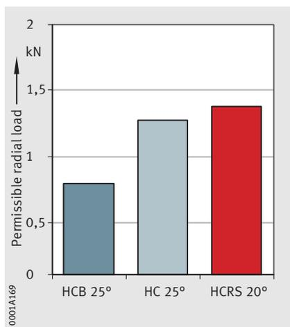
*Figure 6* · Permissible loading under radial load
