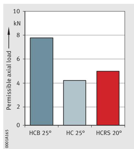
*Figure 5* · Permissible loading under axial load
