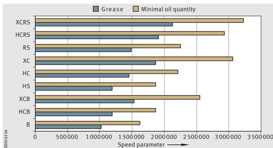
Figure 2 · Comparison – speed parameters
