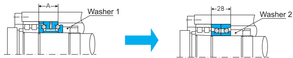
Fig. 5 The mounting of high-speed angular contact thrust ball bearings
