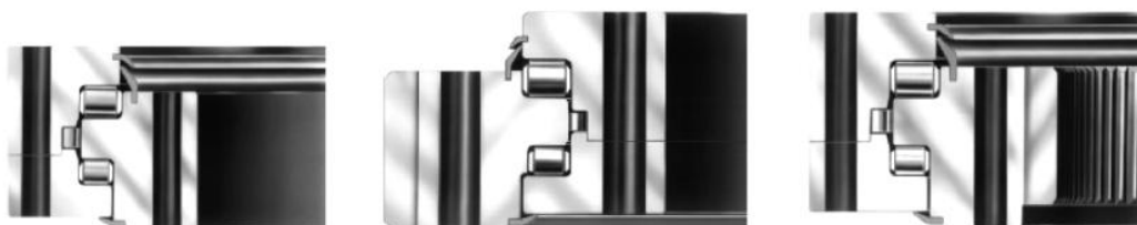
三排圆柱滚子组合转盘轴承 Three row cylindrical roller slewing bearing
