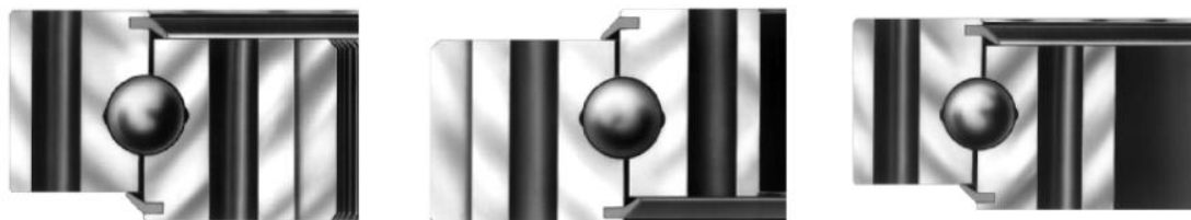
单排四点接触球转盘轴承 Single row four point contact ball slewing bearing
